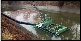
Trash traps do not slow down water or help it to infiltrate. However, they are fairly effective at removing marine debris from rivers and other flowing water as it heads downstream. The litter trap pictured above is just one example. Any trash trap requires the commitment of an organization to continuously remove captured litter. Trash traps can be purchased fully built, but there are also do-it-yourself options.
