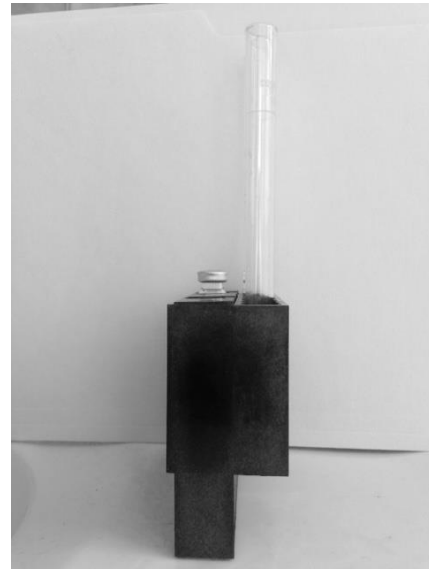
Figure 3: Top edges of Axial Reader and Octet-Comparator are aligned.
