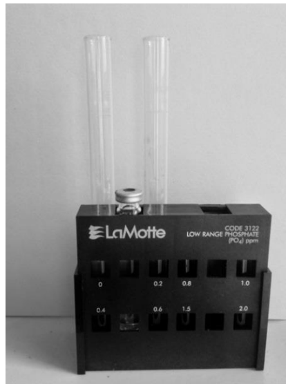
Figure 1: Octet-Comparator with sealed vial of distilled water and two untreated sample test tubes, placed correctly.
