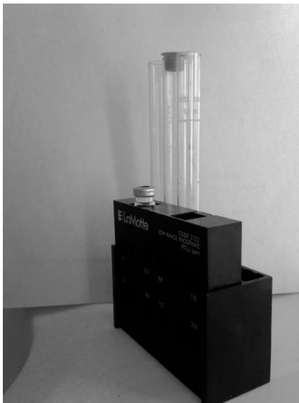
Figure 2: The treated sample has a lid on it, and is placed correctly.
