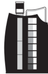
Figure 1 Octa-Slide viewer with Octa-Slide Bar and test tube inserted
